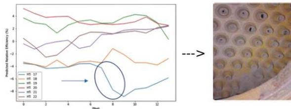
Modelled Truck Efficiency detects clogged air filter on a CAT 793
